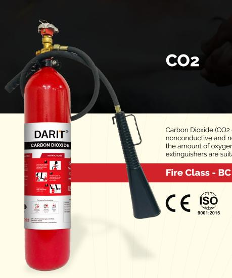
Carbon Dioxide (CO2 extinguishers use the nonconductive and noncorrosive CO2 gas to reduce the amount of oxygen available to the fire. CO2 extinguishers are suitable for Class B and E fires.
